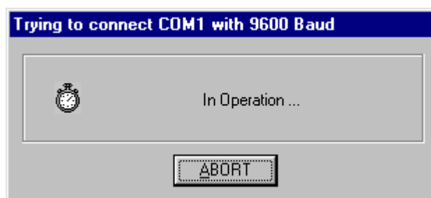
Figure 4-2. Port Scanning at Startup of GUI Software
